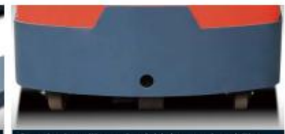
Standard auxiliary wheel, higher truck stability
